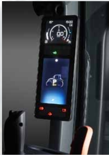
On HiTech and Active models, engine, transmission, hydraulics and other settings are made on the new smart display. On all models, it can be used to display the basic gauges and warning lights, as well as to view information selected by the driver.
