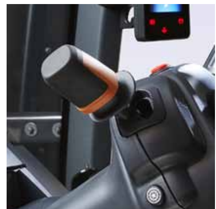
Valtra's forward-reverse shuttle lever has been updated.
