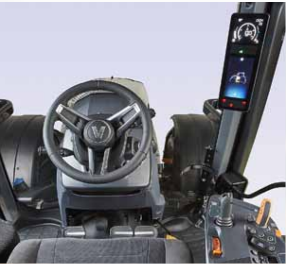
The cab on the new N and T Series has been thoroughly revamped. The instrument cluster has moved from the steering column to the A pillar, where it is clearly visible. The approximately 40 centimetre high smart display is operated from below the steering wheel.
