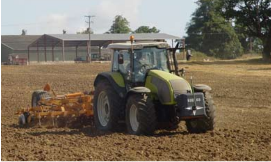
The excellent traction, high PTO power and low weight of the T190 is ideal for preparing potato ground
